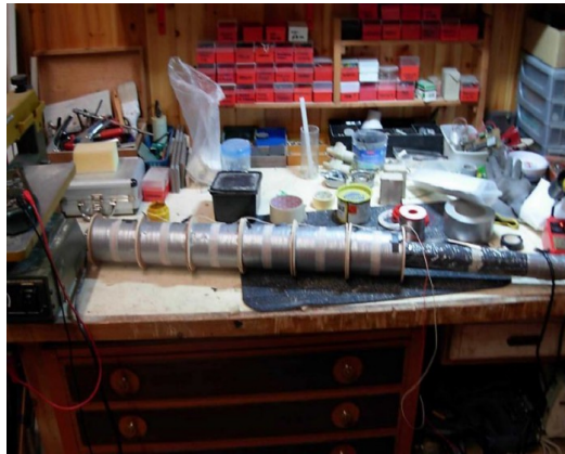
Fig. 6 Realisation of the antenna with very high inductance Note the 6 coils with 17,000 turns of insulated copper wire and the protruding core formed by soft iron bars.
